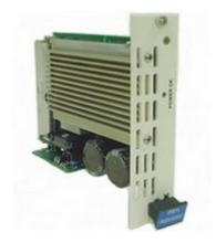
110/220Vac Input, 100W Single +5Vdc Output
