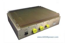
Single Phase 60Hz 115/220Vac Primary Input +24Vdc Secondary Input (Backup Battery) Dual Output, +28Vdc and 115Vac, 335W Max Total
